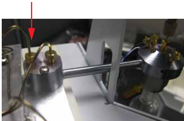
Figure 5-64 Purge Valve Normally Open (NO) tubing to the 4-Way Tee
