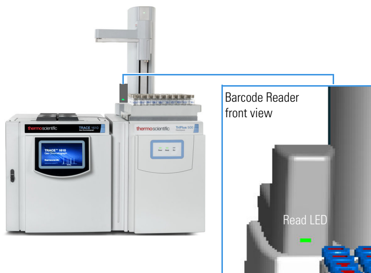
Figure 63. Barcode Reader Installation (4)
