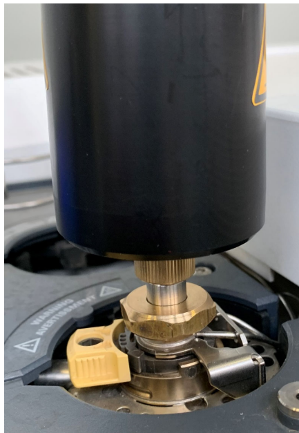
Figure 35. Transfer Line Installed to GC Adapter
