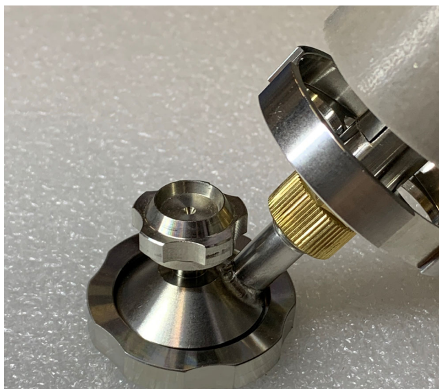
Figure 28. SSL Adapter Connected to the TriPlus 500 HS Transfer Line
