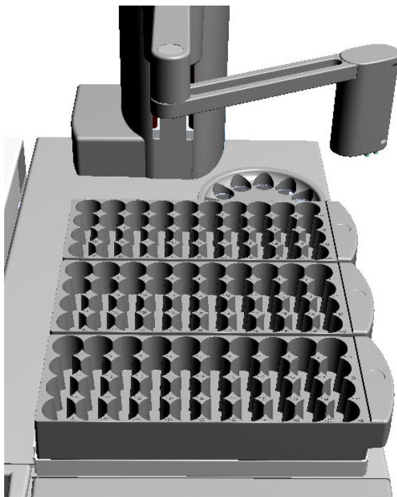
Figure 57. Vial Tray Installation on TriPlus 500 HS (6)
