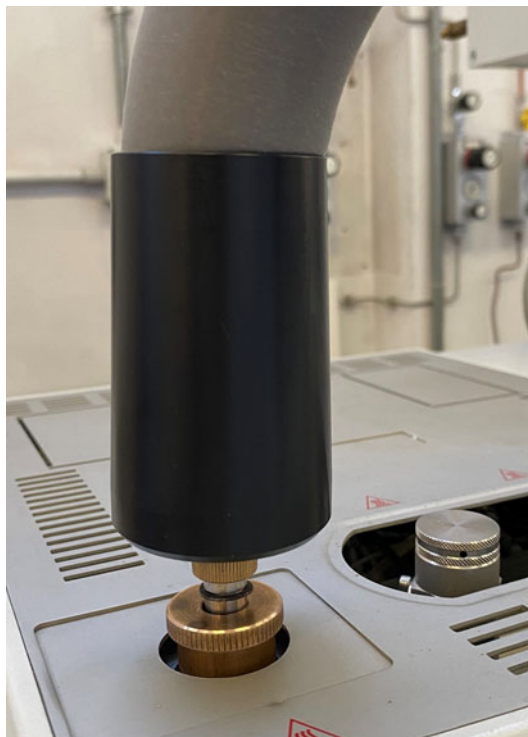
Figure 38. Transfer Line Connected to the TRACE GC Ultra SSL Inlet
