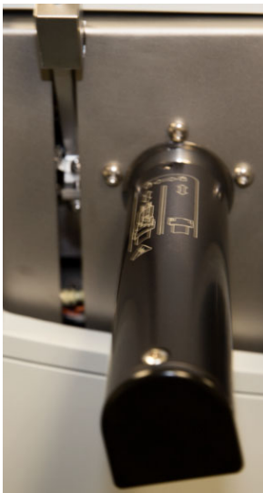
Figure 20. V-lock Source Plug Inserted Correctly
