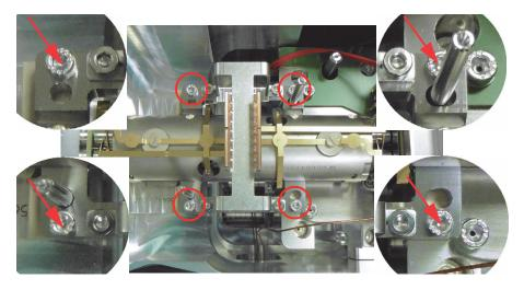
Figure 8-42. Quadrupole screws
