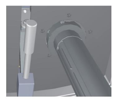
**Figure 8-5.** Inserting the Ion Volume Tool
