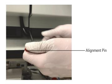
**Figure 5-6.** Securing the GC to the MS with the Alignment Pin
