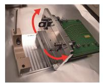
**Figure 8-45.** Releasing the bent flatapole exit lens
