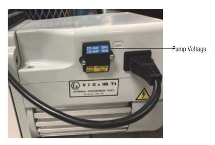
**Figure 5-13.** Confirming the Pump Voltage
