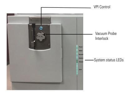
**Figure 3-1.** Orbitrap Exploris GC and Orbitrap Exploris GC 240 MS front view
