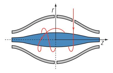
Figure 3-14. Schematic of Orbitrap cell and example of stable ion trajectory
