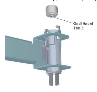
**Figure 8-19.** Inserting Lens 2 into the Source Sleeve
