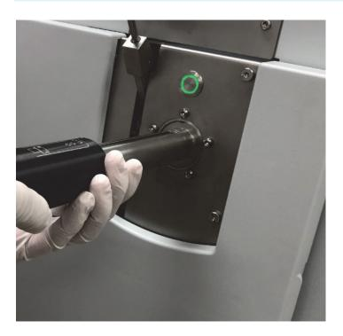
**Figure 8-8.** Pushing the Tool into the Instrument
