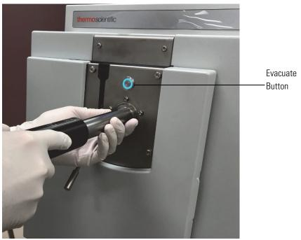
Figure 8-27. Evacuating the Instrument
