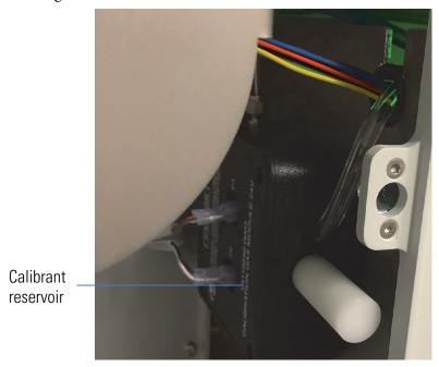
Figure 8-32. Locating the Calibrant Reservoir
