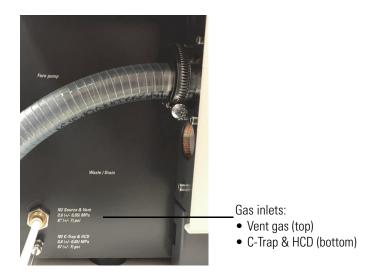
Figure 5-16. Gas connections at the left instrument side
