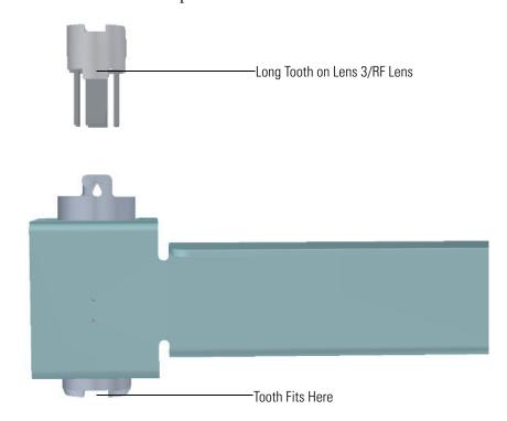
Figure 8-18. Inserting Lens 3/RF Lens into the Source Sleeve
