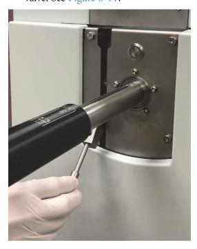
Figure 8-11. Pulling Down the Vacuum Interlock Handle
