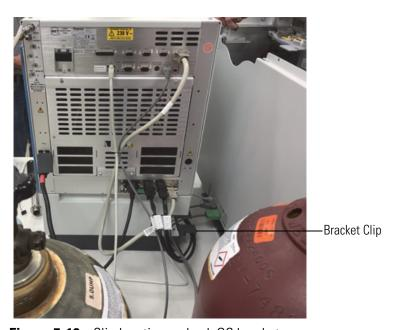
Figure 5-10. Clip location on back GC bracket
