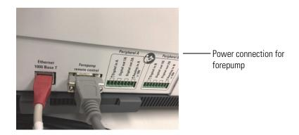
**Figure 5-14.** Power connection for forepump on Orbitrap Exploris GC MS
