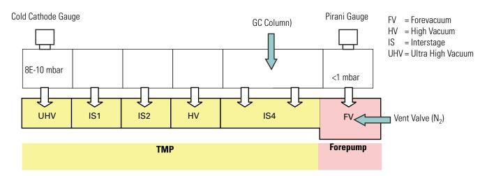
Figure 3-17. Schematic of vacuum system in Orbitrap Exploris GC and Orbitrap Exploris GC 240 MS
