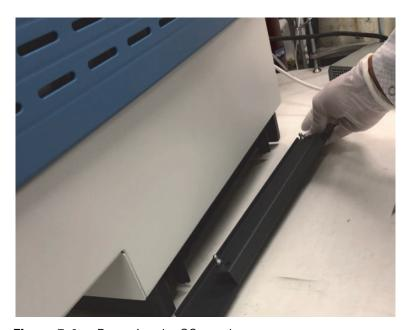
Figure 5-4. Removing the GC panel
