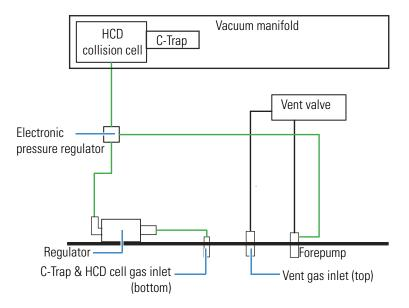
**Figure 3-4.** Schematic of the internal gas supplies
