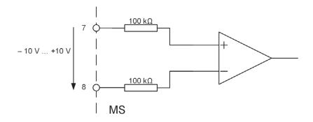
Figure 5-21. Analog input equivalent schematic
