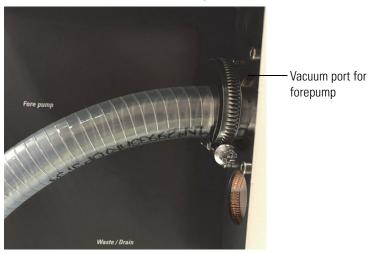
Figure 5-12. Vacuum port of Orbitrap Exploris GC MS
