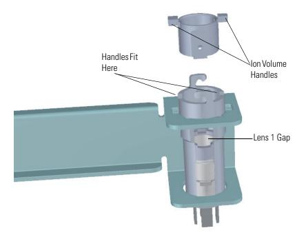
**Figure 8-21.** Inserting the Ion Volume into the Source Sleeve
