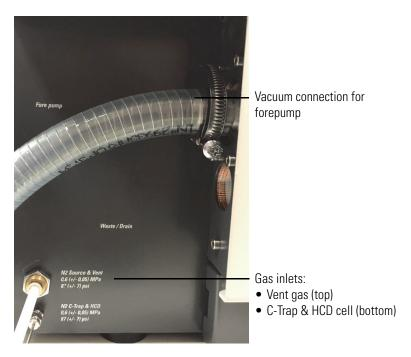
**Figure 3-3.** Connections at the left instrument side
