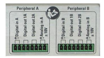
Figure 5-18. Peripheral control connectors
