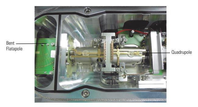
Figure 8-41. Inside of quadrupole chamber (customer accessible parts)
