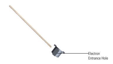
Figure 8-31. Cleaning the CI Ion Volume
