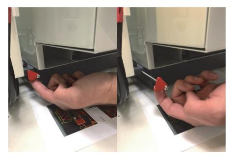
Figure 8-36. Removing the alignment pin
