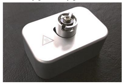
**Figure 6-4.** Attaching the Source Plug to the Source Plug Holder
