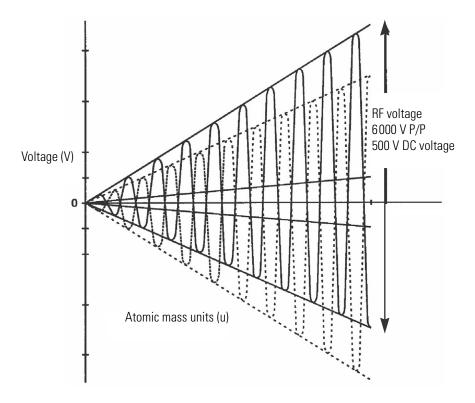
**Figure 3-13.** Magnitude of the RF voltages and DC voltages applied between the rods of the quadrupole mass filter
