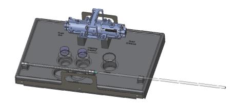
Figure 8-48. Quadrupole mounted on holder
