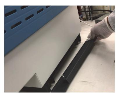
Figure 8-37. Removing the GC panel
