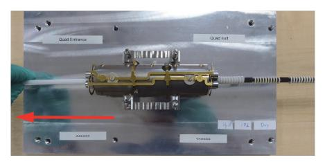
Figure 8-51. Cleaning the quadrupole
