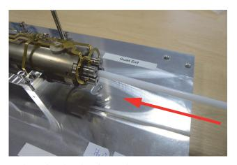
Figure 8-50. Inserting the cleaning tool
