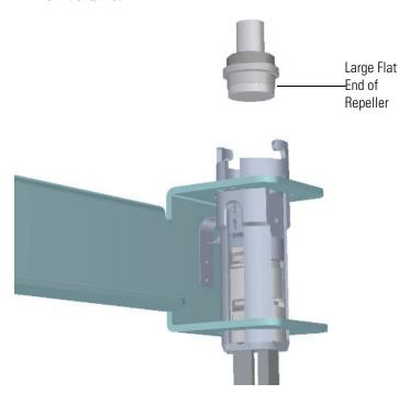
Figure 8-22. Inserting the Repeller
