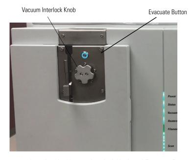
**Figure 8-3.** Locating the Vacuum Interlock Knob and Evacuate Button
