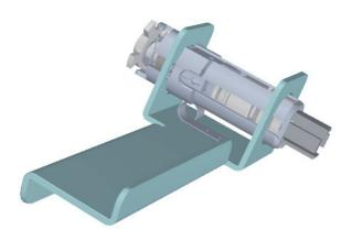
**Figure 8-15.** Removing the Ion Source Cartridge
