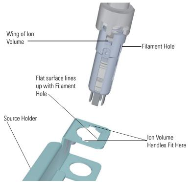
Figure 8-14. Attaching the Source Holder
