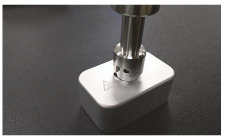
**Figure 6-5.** Attaching the Source Plug to the Source Exchange Tool
