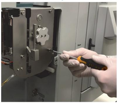
Figure 8-34. Loosening the Manifold Screws
