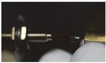
**Figure 6-10.** Inserting the New Column through the MS Transfer Line
