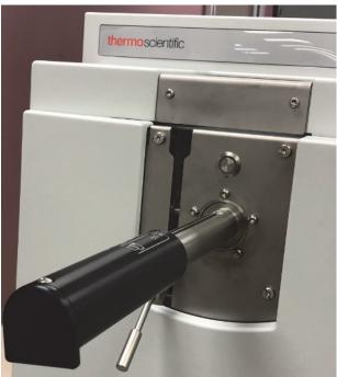
Figure 8-30. Pulling Down the Vacuum Interlock Handle
