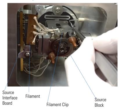
Figure 8-35. Loosening the Filament Clip from the Source Block
