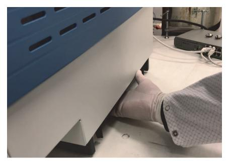
Figure 5-5. Taking off the GC brakes
