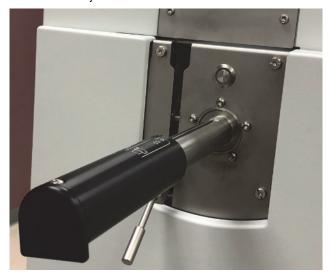
**Figure 6-7.** Inserting the Source Plug into the Vacuum Interlock
