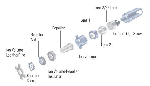
**Figure 8-16.** Components of the Orbitrap Exploris GC and Orbitrap Exploris GC 240 Ion Source
