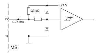
Figure 5-20. Digital In input equivalent schematic
