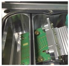
**Figure 8-44.** Sliding out the bent flatapole
