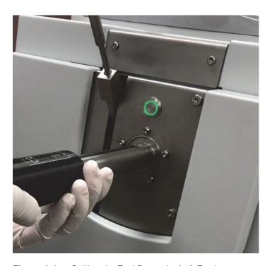
Figure 8-9. Pulling the Tool Down the Left Track
