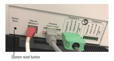
**Figure 6-1.** System reset button on control panel
