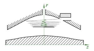
**Figure 3-15.** Principle of electrodynamic squeezing of ions in the Orbitrap analyzer as the field strength is increased
