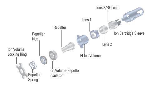
Figure 3-10. Components of the Orbitrap Exploris GC Ion Source
