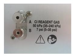
**Figure 5-17.** Connecting the Cl gas supply
