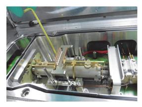
**Figure 8-53.** Reinstalling the quadrupole
