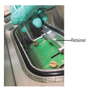
**Figure 8-43.** Loosening the screws of the bent flatapole
