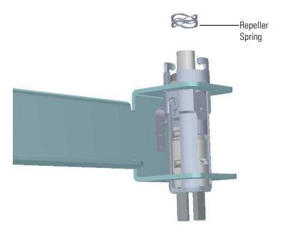
Figure 8-23. Inserting the Repeller Spring into the Sleeve
