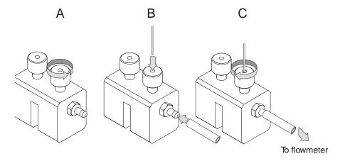
**Figure 6-2.** Connecting the Column to the Flowmeter
