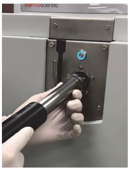
**Figure 8-12.** Removing the Tool from the Instrument
