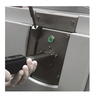
**Figure 8-10.** Locking the Tool in Place. Note: Tool is Rotated Left.
