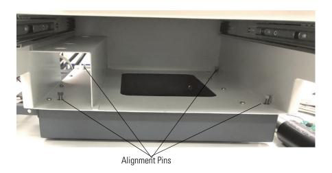
Figure 5-7. Leveling the GC with the alignment pins
