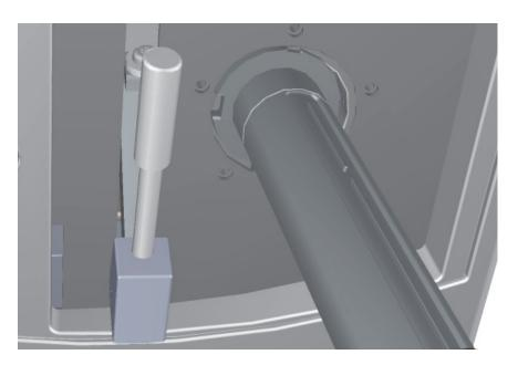
Figure 8-6. Twisting the Tool into Place
