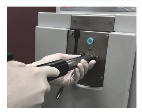
Figure 8-28. Pushing the Tool into the Instrument
