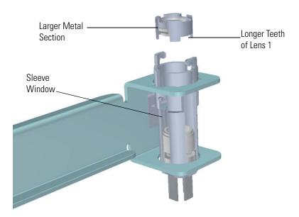
Figure 8-20. Inserting Lens 1 into the Source Sleeve
