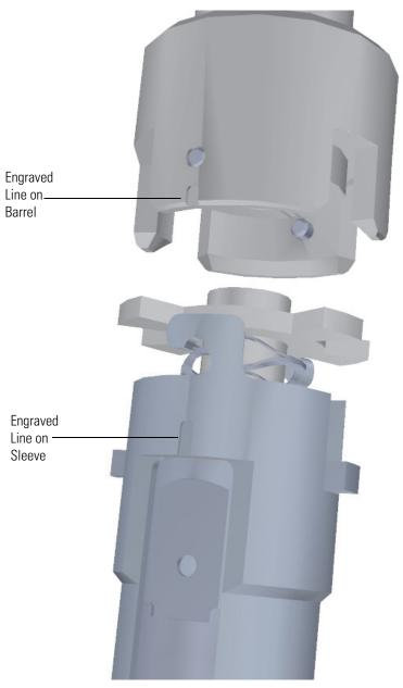
Figure 8-25. Aligning the Tool with the Ion Source Cartridge
