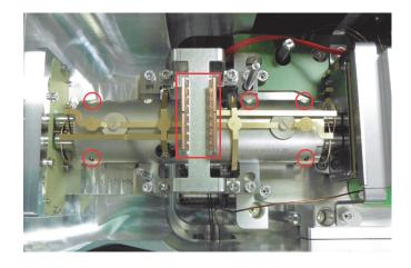
**Figure 8-52.** Checking the quadrupole seating
