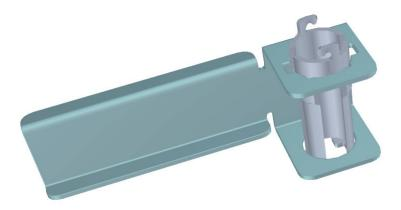
Figure 8-17. Inserting the Sleeve into the Source Holder
