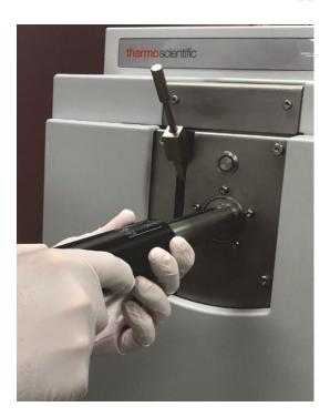
Figure 8-29. Pulling the Tool Down the Right Track
