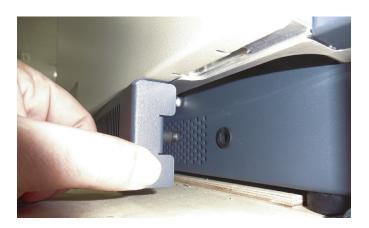
**Figure 8-2.** Removing a fan filter bracket
