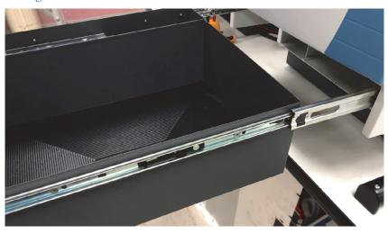
**Figure 5-8.** Sliding the drawer into the GC riser
