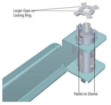
**Figure 8-24.** Inserting the Locking Ring into the Sleeve
