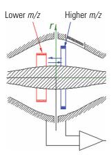
**Figure 3-16.** Approximate shape of ion packets of different *m/z* after stabilization of voltages
