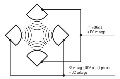
**Figure 3-12.** Polarity of the RF voltages and DC voltages applied to the rods of the quadrupole mass filter
