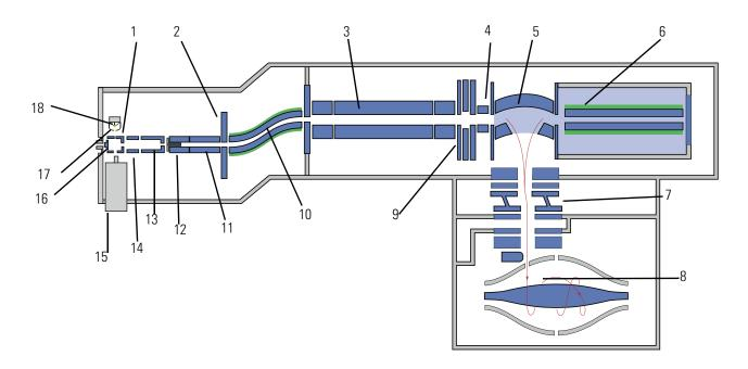
Labeled Components: 1=Ion Volume; 2=Inter Flatapole Lens; 3=Quadrupole; 4=Transfer Multipole; 5=C-Trap; 6=HCD Collision Cell; 7=Z-lens; 8=Orbitrap Mass Analyzer; 9=Independent Charge Detector; 10=IBent Flatapole; 11=Injection Flatapole; 12=Lens3/RF Lens; 13=Lens 2; 14=Lens 1; 15=Transfer Line; 16=Repeller; 17=Electron Lens; 18=Dual Filament
