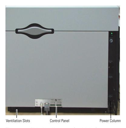
**Figure 3-5.** Right side of instrument (partial view)
