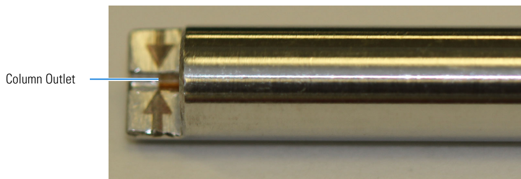
Figure 6. Lining Up the Column in the Column Measuring Tool
