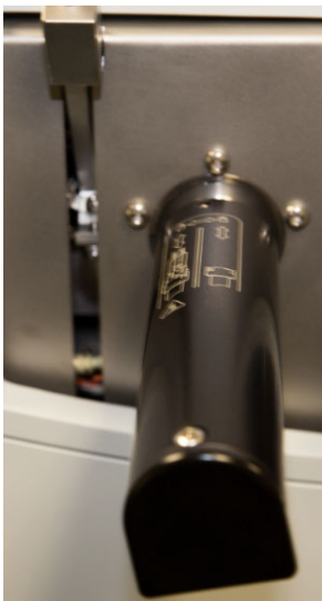
Figure 20. V-lock Source Plug Inserted Correctly
