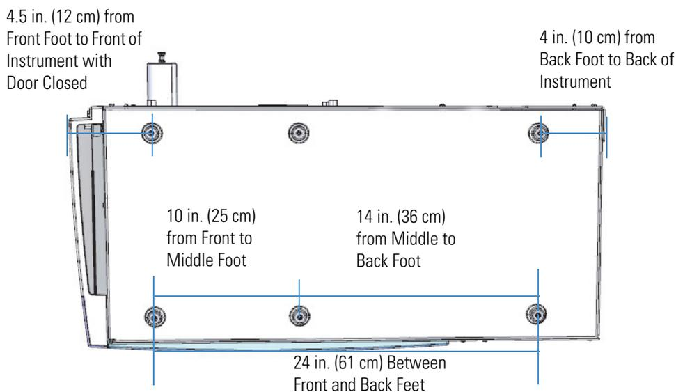
**Tip** Thermo Fisher Scientific requires that all six of the instrument's feet be positioned on a bench. Overhang of the front, the back, or both ends of the instrument off the bench front or back is acceptable. If the depth of your bench is less than the distance between the factory-installed feet, please contact the factory ([usaus.gcms.licensing@thermofisher.com](mailto:usaus.gcms.licensing@thermofisher.com)) for your other options of positioning the instrument on such a narrow bench.
