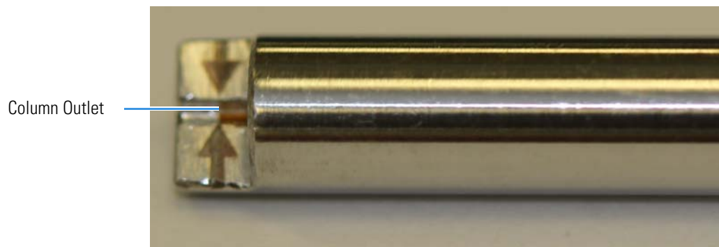
Figure 26. Line up the outlet of the column with the arrows on the end of the column measuring tool. Lining Up the Column in the Column Measuring Tool
