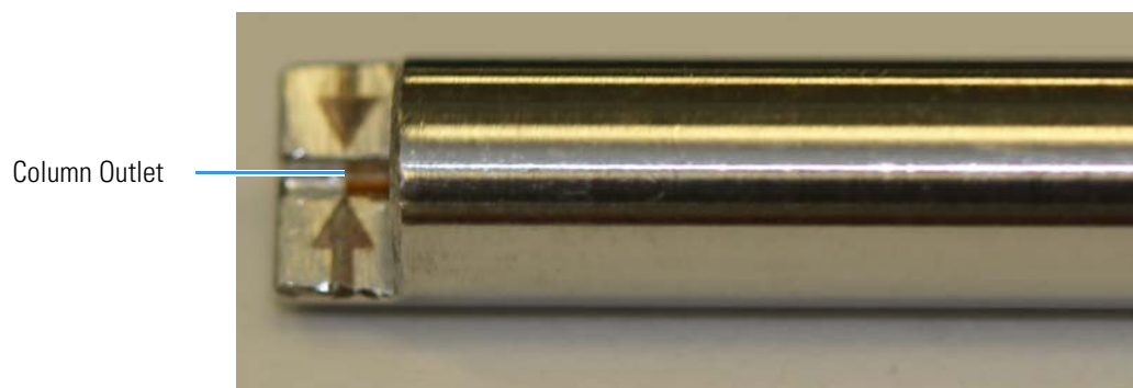
Figure 19. Lining Up the Column in the Column Measuring Tool
