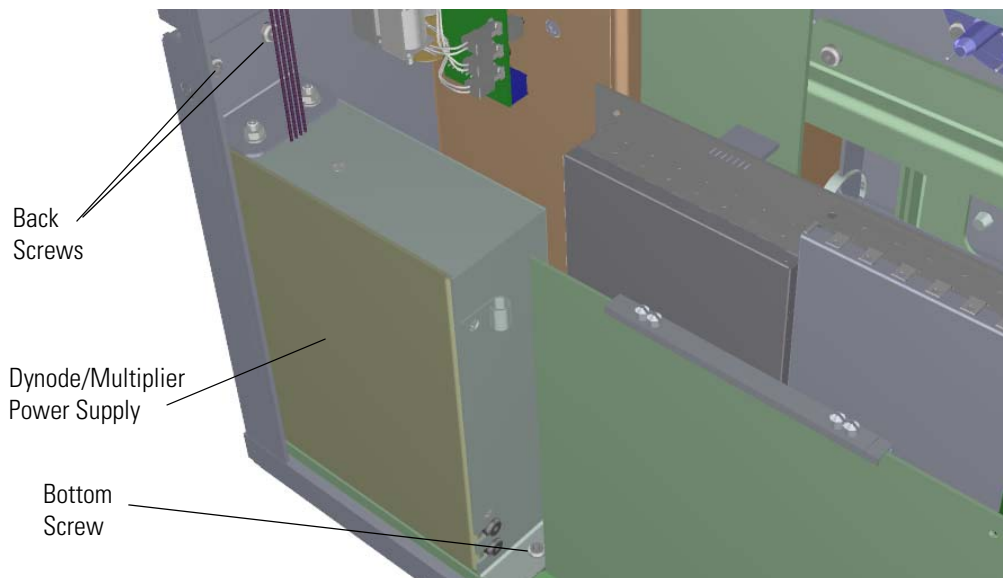
Figure 366. Removing the Dynode/Multiplier Power Supply
