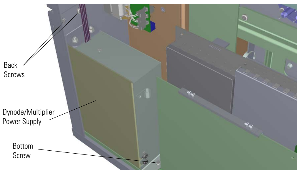
Figure 384. Reinstalling the Dynode/Multiplier Power Supply
