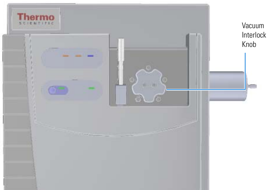
Figure 46. Removing the Vacuum Interlock Knob
