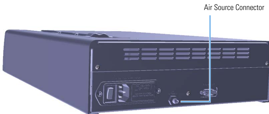
Figure 6. Connecting the Air Source to the Direct Probe Controller
