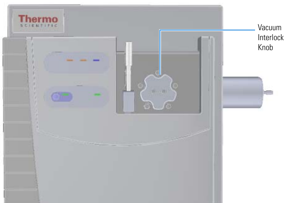
Figure 62. Reattaching the Vacuum Interlock Knob
